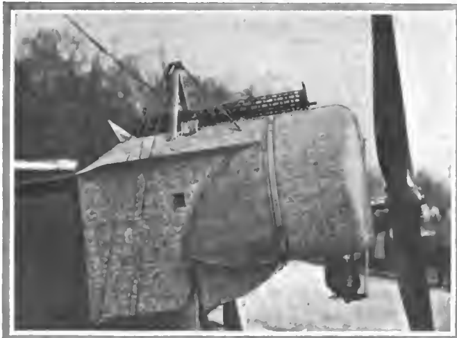
Engine housing and machine gun on captured Fokker monoplane. Engine is a rotary Oberursel like the French Gnome
